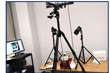
Vibration experimental setup with the DIC system
