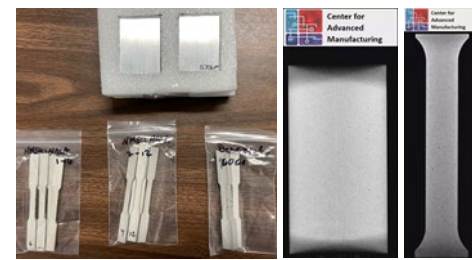
First set of AlSi10Mg specimens manufactured using a reference set of AM DED parameters and characterized using X-Ray CT at Navajo Tech
