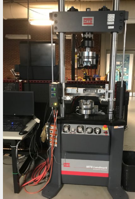
MTS Landmark Machine Capacity: 100 kN
