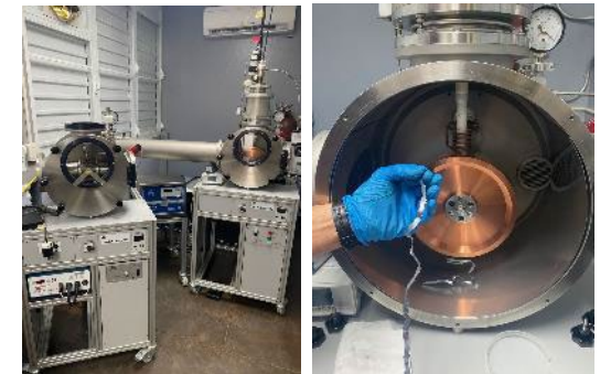
Left: Ultra rapid splat quencher and melt spinner. Right: Rapidly solidified Al-Ce ribbon.
